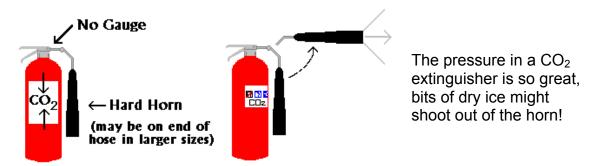
$CO_2$  cylinders are red. They range in size from 5 pounds to 100 pounds or larger. On larger sizes, the horn will be at the end of a long, flexible hose.
